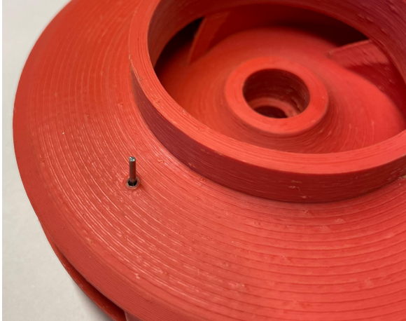
Figure 5: Unbalance mass place.
