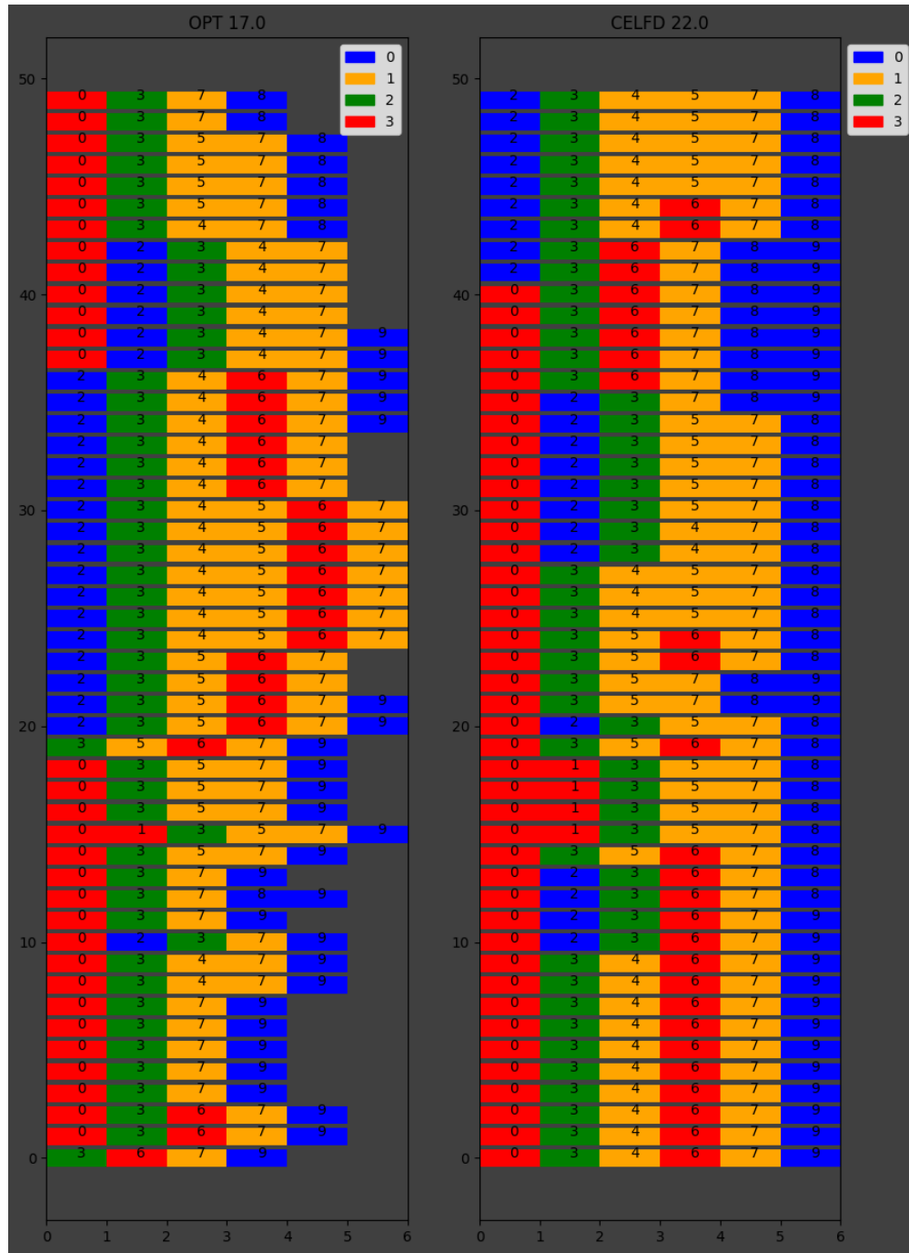
Figure 2.1: On the left, we have the optimal schedule for the instance presented, where the colors of each page are represented by the colors of the blocks, and the page is represented with the number inside the rectangle. The initial cache is on the bottom, while the final cache is on top, above this, we can see the cost for the algorithm. On the right, we have the schedule for the CELFD algorithm, with the same plot structure.
